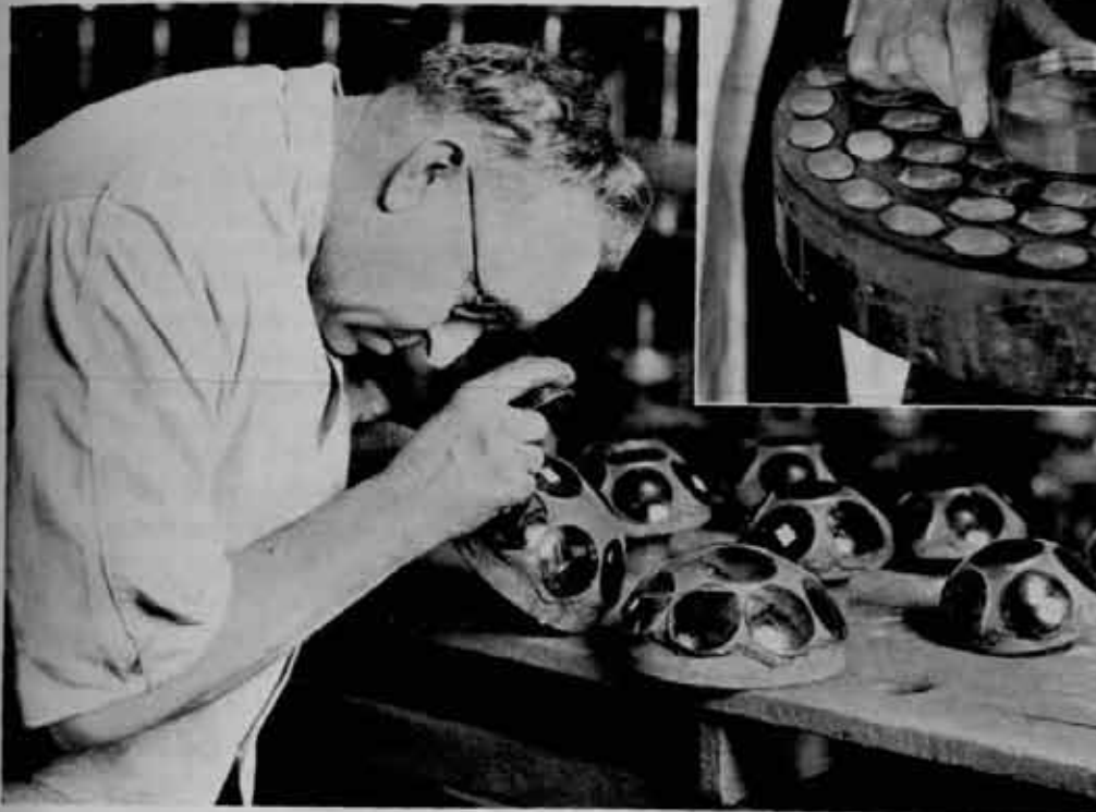
The most critical inspection known to optical science—testing prisms by means of Newton's rings and light rays—accurate to millionths of an inch.
