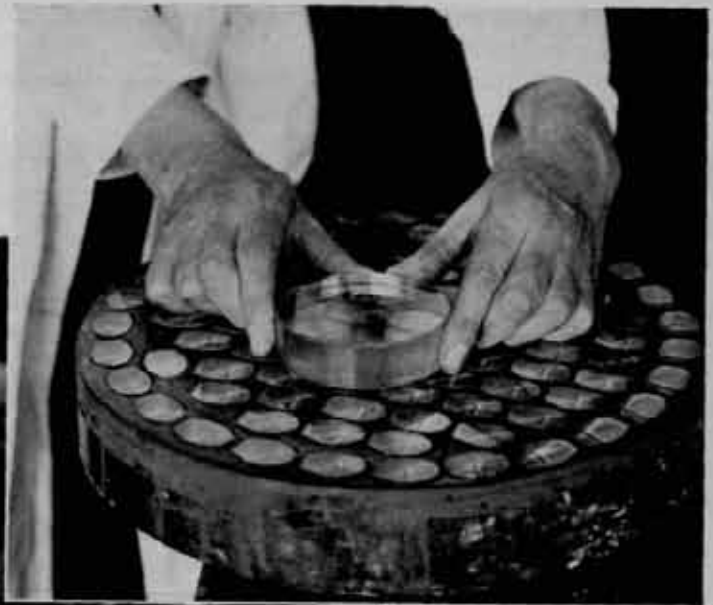
Inspecting polished lens surfaced on a shell, or form, of specified curvature
