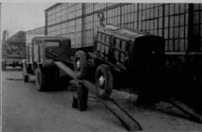
Right—Loading power plant into standard cargo truck.
